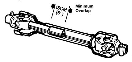
G. Clamp end of driveline in a vice. Cut off shield where marked. (Figure 2-3).
